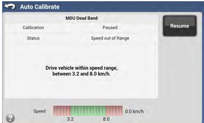
Figure 3-57 MDU Dead Band Calibration
