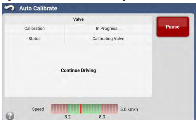
Figure 3-55 Valve Calibration in Progress
