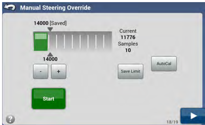
Figure 3-21 Manual Steering Override Adjustment (Hydraulic)
