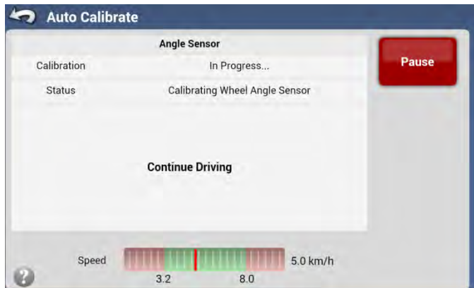
Figure 3-54 Angle Sensor Calibration in Progress
