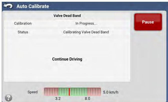
Figure 3-53 Dead Band Calibration in Progress
