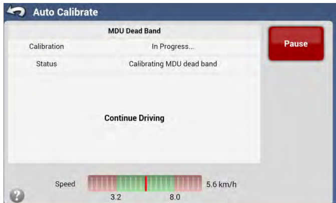
Figure 3-58 MDU Dead Band Calibration in Progress
