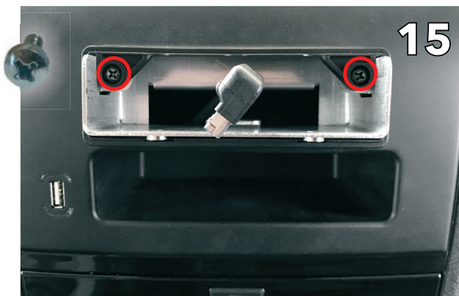
Put the fascia in (make sure to connect the USB on the panel) and tighten with 2 screws
