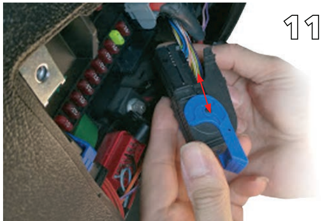
Remove the black connector and slide open
