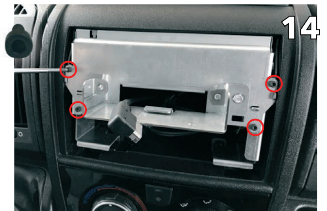
After installing the interface, slide the unit into the dashboard, routing the display cable underneath and tighten 4 small allen screws
