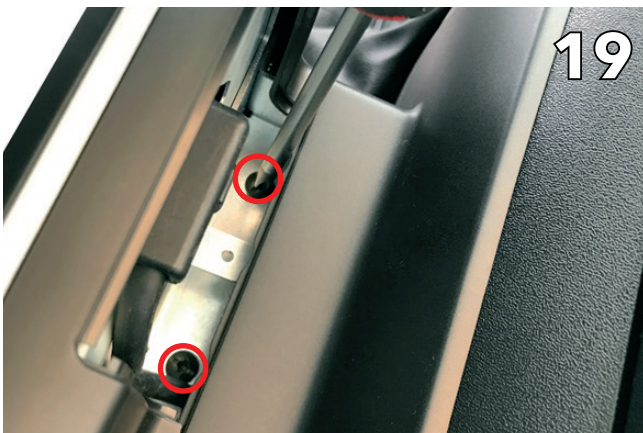
Slide the screen into the dashboard and tighten with 2 screw from the top
