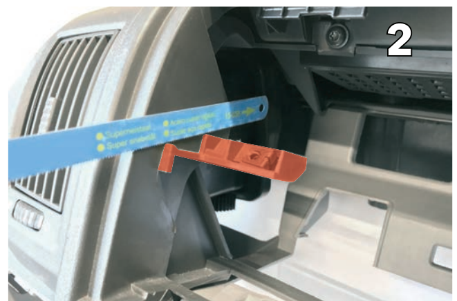
Cut out the center supports / support bar
