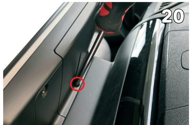
Make sure the display connector is plugged in and put the cover over it - Secure with one screw
