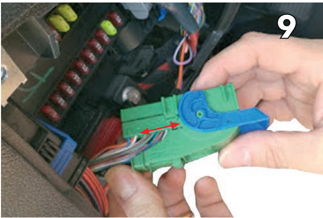
Remove the green connector and slide open
