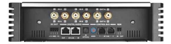
The input panel of TH amps features AD Link connectors, dedicated to receiving the digital signal from Audison bit sources or processors and relaunch it towards the amplifier chain in Full DA HD configuration, through a shielded Cat.5 cable provided with an RJ45 connector.
