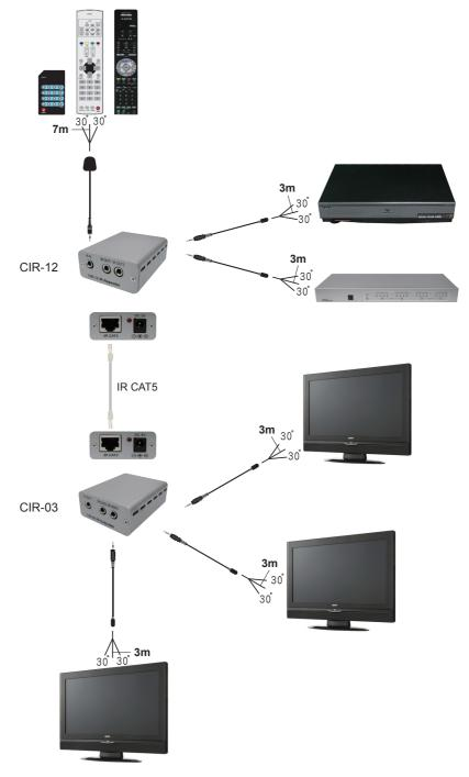
Note: A. IR receiver's control distance can goes up to 7 meters long with open space and direct angle.
