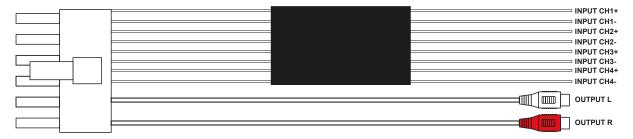
The **OUTPUT** RCA jacks of both wire harnesses provide a linear full-range audio signal for driving additional amplifiers.
