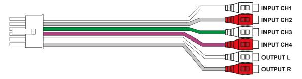
If your head unit does not have RCA preamp outputs, you can use the amplifier's high level inputs as signal input. Make sure that the **INPUT LEVEL** push-button (# 7) is in the **HIGH** position (pushed). Simply connect the loudspeaker cables of the head unit to the enclosed wire harness as follows:
