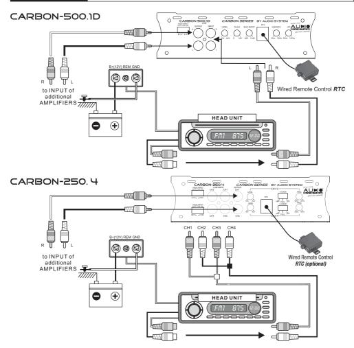
The **CARBON-SERIES** amplifier offers RCA-Inputs, which are connected through cinch cables with the preamplifier-outputs of the head unit. If the head unit (OEM-RADIO) has no RCA-Output, then it is possible to connect the speaker output direct to High-Input of the amplifier.
